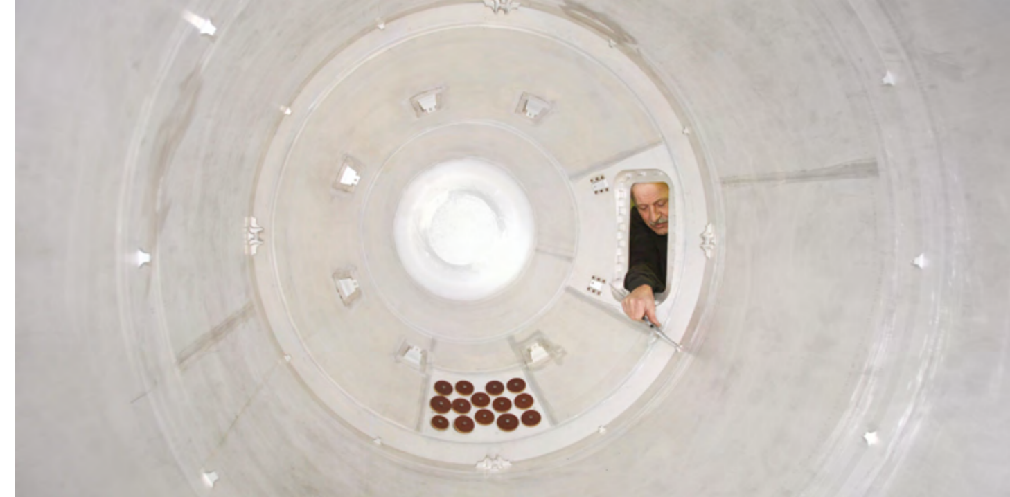
An engineer takes measurements inside the metal body of a Russian GLONASS positioning satellite at the Applied Mechanics Institute in Zheleznogorsk, Russia.
